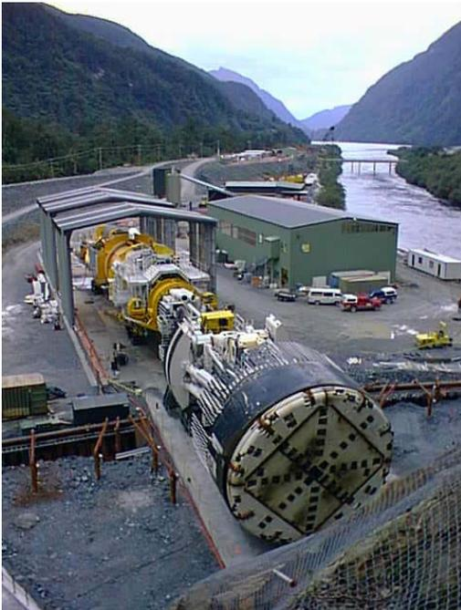
Tunnel boring machine and back-up system in front of the portal
